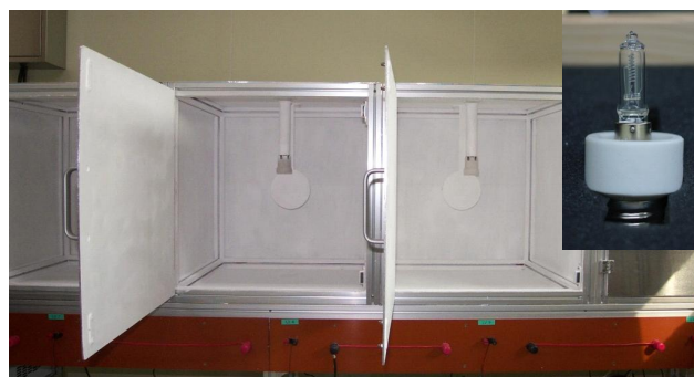
Figure 2. The pre-burning facility for 150 W E11-based lamps consisting of 5 partitions for 5 individual lamps. The inner surface is white-painted to monitor the spatially averaged photometric output imitating an integrating sphere. A baffle is placed in-between a photometer and a lamp.
