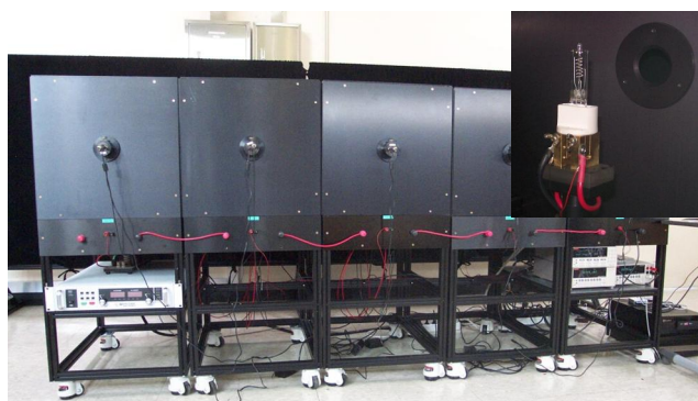
Figure 1. The pre-burning facility for 1 kW FEL-type lamps consisting of 5 partitions for 5 individual lamps.
