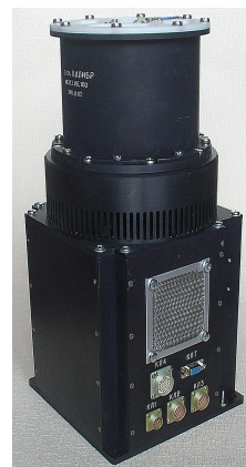
Figure 1. The gallium onboard fixed-point BB prototype "KALIBR" tailored for space experiment.
