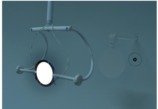
Figure 1. Photograph of the new 2-axis OLED holder. Panel 1 was attached for efficacy measurement.
