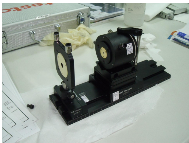
Figure 3. Radiancemeter (Si trap detector plus two precision apertures at a fixed distance) used to calibrate the FIRA in absolute spectral response.
