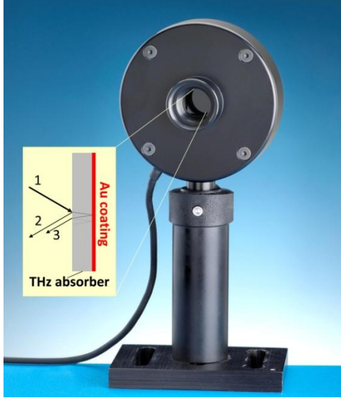
Figure 3. Photo of the new THz detector standard. The cutaway view exhibits a schematic cross-section of the THz radiation absorber with a gold (Au) coating on its back side.
