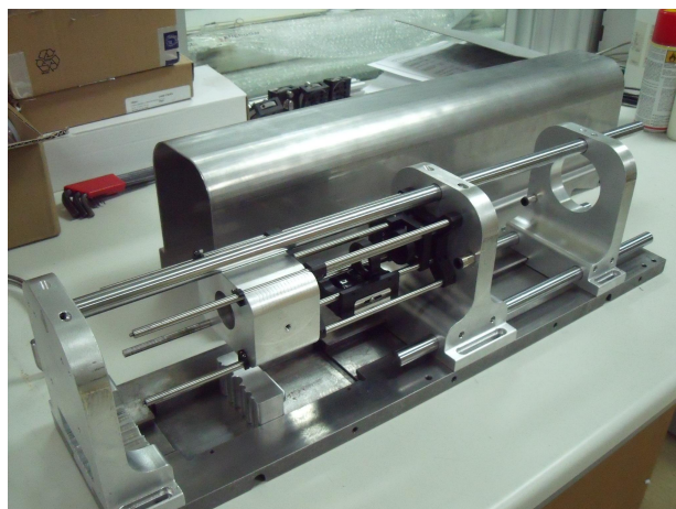
Figure 2. Picture of the FIRA. It is 65 cm long and 18 cm high. It weights 30 kg.
