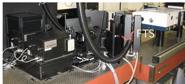
Figure 1. Setup with the monochromator system on the left. Its monochromatic and parallel beam enters the FTS that stands on the right optical table at the place where usually the detectors (e.g. solar cells) were mounted.
